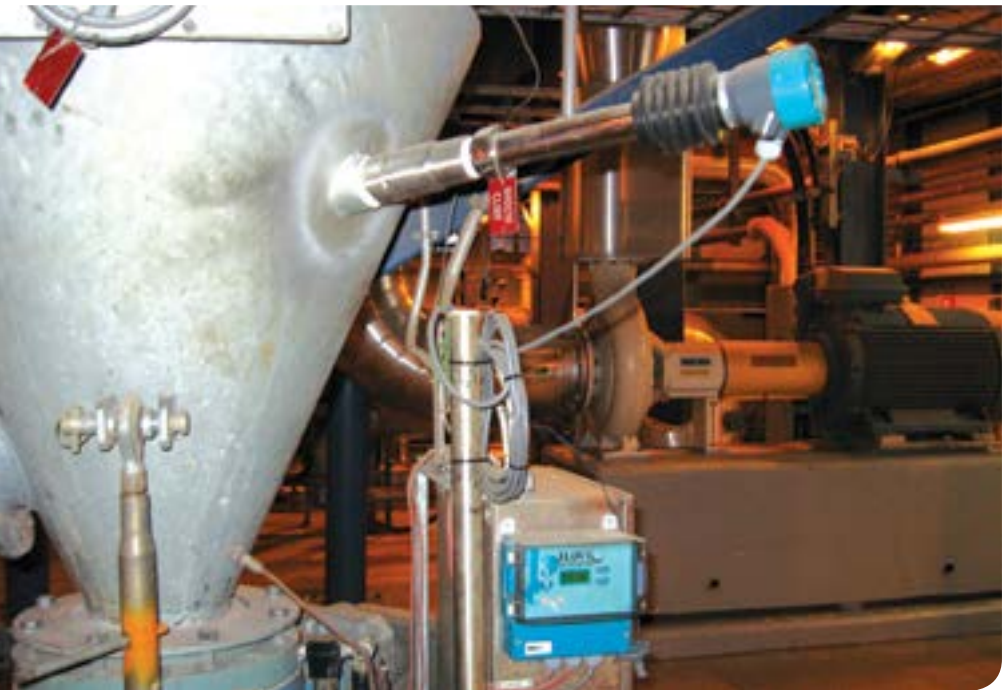
High and Low Level Switch In A Hopper
