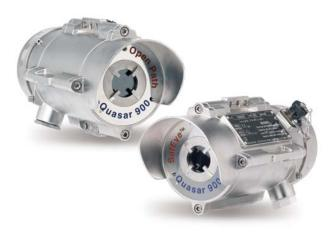
The Quasar 900 consists of a Xenon Flash infrared transmitter and infrared receiver, separated over a line of sight from 23 ft (7m) up to 650 ft (200m) in extremely harsh environments where dust, fog, rain, snow or vibration can cause a high reduction of signal.
