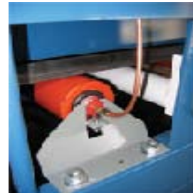
Optional pulley and idler lubrication manifold mounted external to the enclosure
