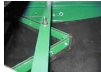
Option "V-Plow" prevents material from building up on underside of belt
