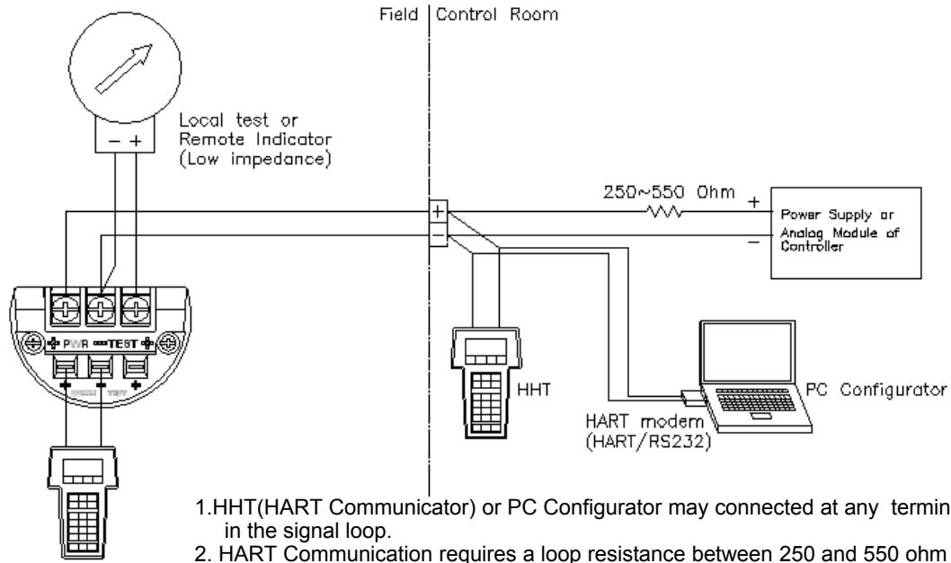
1. HHT(HART Communicator) or PC Configurator may connected at any termination point in the signal loop.
