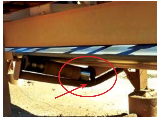
Idler Shell Collapse
