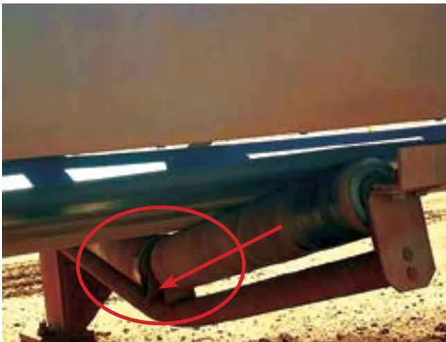
Idler Shell Collapse
