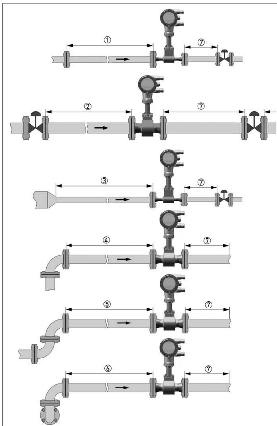
Figure 3-5: Inlet sections
