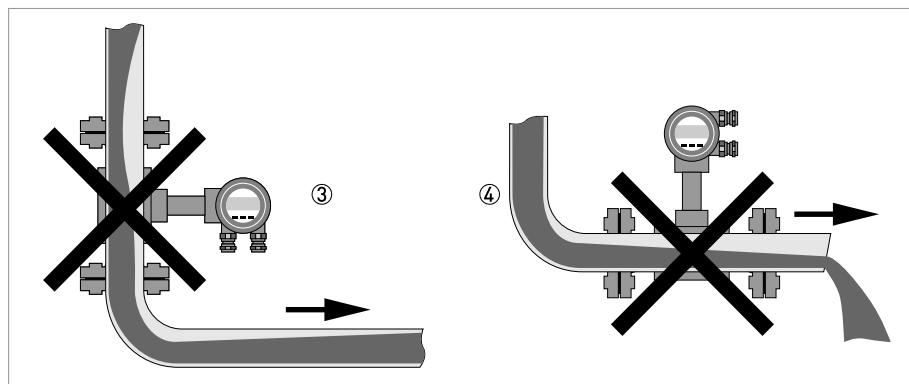
Figure 3-3: Downpipe and outlet
