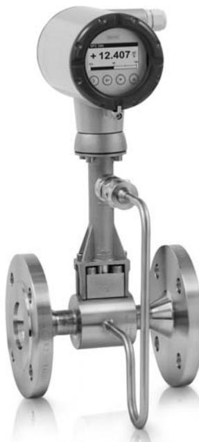
The **OPTISWIRL 4200** with integrated nominal diameter reduction up to two nominal diameter sizes assures best results in accuracy and optimal measuring ranges even in pipelines with large diameters, which have been designed for a low pressure loss.
