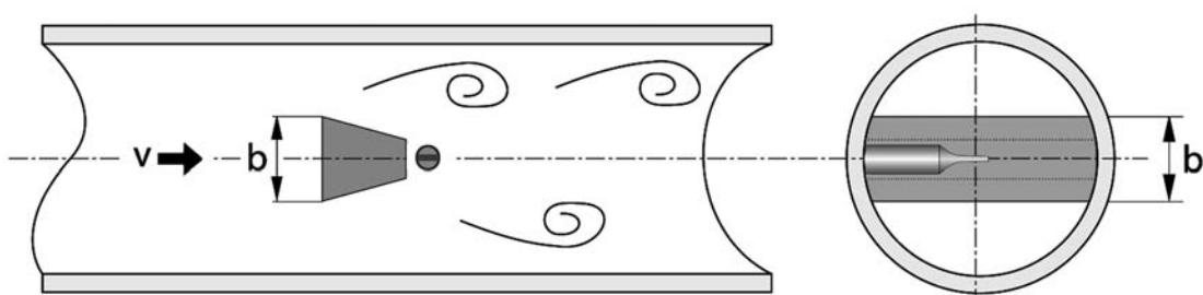
Figure 1-1: Functional principle
