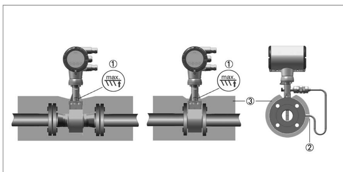
Figure 3-4: Installation heat insulation
