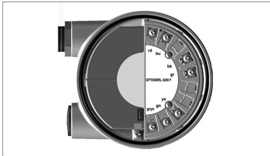
The connections in the sensor and wall mount bracket connection boxes are identical in construction.
