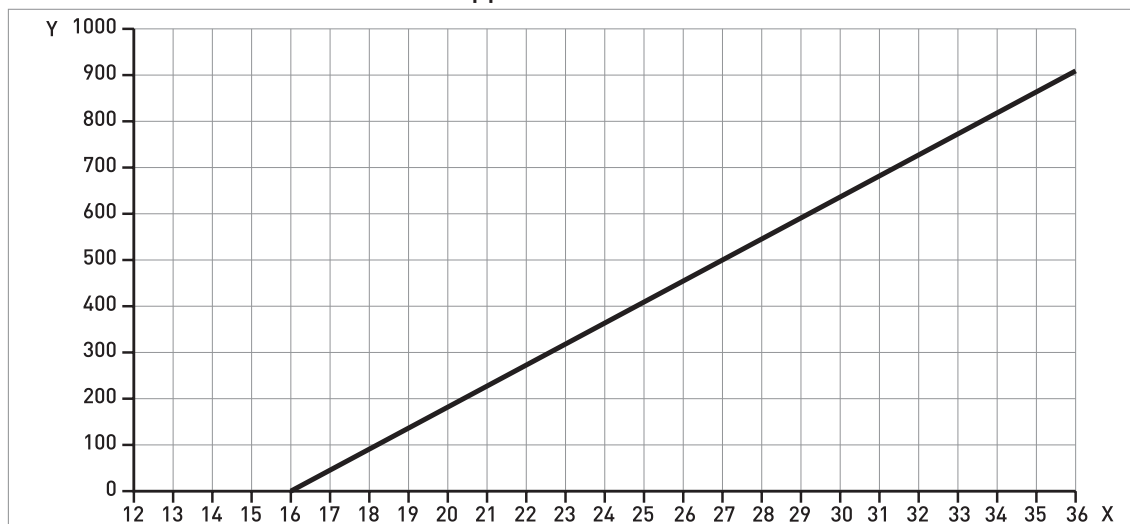
Figure 2-2: Minimum power supply voltage for an output of 22 mA at the terminal (Hazardous Location approval (Ex d / XP/NI))
