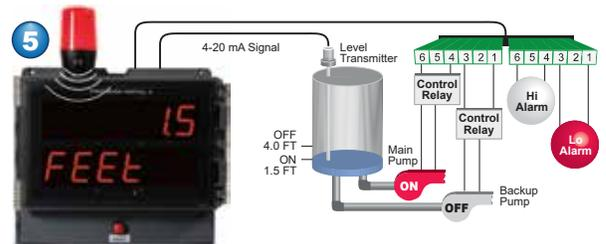
Relay #4 trips the Low-Level Alarm at 1.5 feet and resets at 4.0 feet. The optional light starts flashing and the horn sounds.
