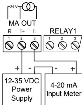
4-20 mA Output Powered by External Power Supply
