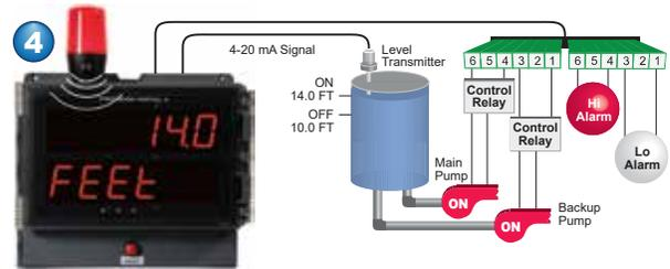
Relay #3 trips the High-Level Alarm at 14.0 feet and resets at 10.0 feet. The optional light starts flashing and the horn sounds.
