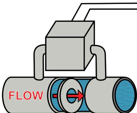
In this application, the PD2-6000 is displaying flow rate by extracting the square root from the 4-20 mA signal from a differential pressure transmitter. The user selectable low-flow cutoff feature gives a reading of zero when the flow rate drops below a user selectable value.
