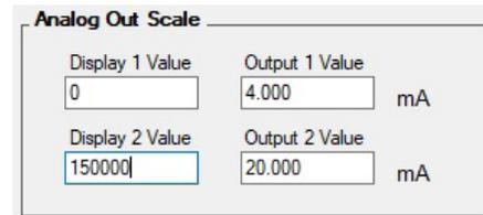
The meter can be set up for reverse scaling as shown below: the output will be 4.00 mA when the display reads 150000 and the output will be 20.00 mA when the display reads 0.
