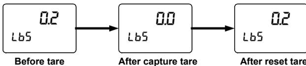
Reset tare removes the display offset of the net value, and the gross and net values become the same until a new capture tare is entered.
