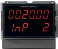
The Helios is prompting for the value for Input 2 and displaying the default value of 20.00 mA. The "2" in 20.00 is brighter than the rest of the digits indicating that it is the number that will be changed by the Up and Right arrows.
