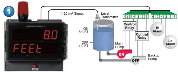
Relay #1 turns the main pump on at 8.0 feet and turns it off at 4.0 feet.
