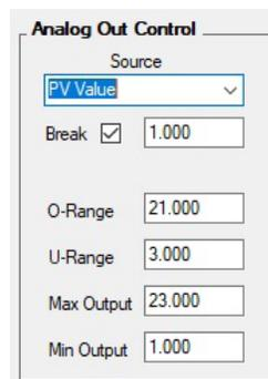
**Source:** Source for generating the 4-20 mA output (e.g. PV)
