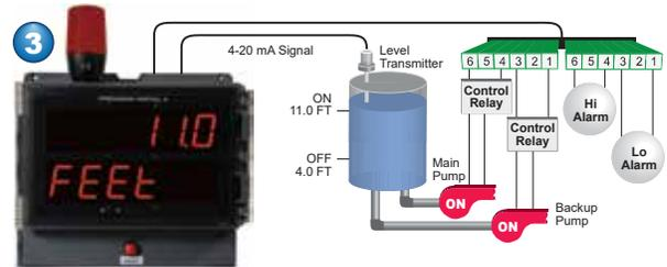
If the backup pump is not able to keep up, and the level reaches 11.0 feet, relay #1 transfers and starts the main pump as well.
