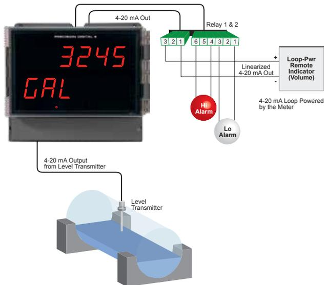
In this application, a level sensor is measuring the height in the round horizontal tank and the Helios is converting that signal to volume using the RHT function. All the user has to do is input the diameter and length of the tank and the meter converts the signal to volume.
