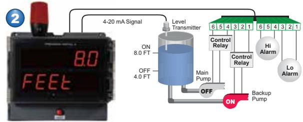
With the Pump Alternation feature activated, the next time the level reaches 8.0 feet, relay #2 transfers and starts the backup pump.
