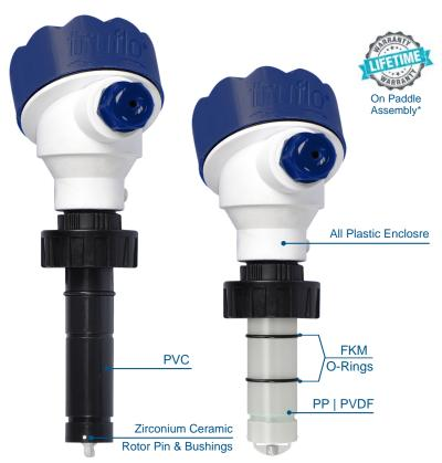
The TIR digital flow meters are easy to install with exceptional long life performance. Truflo TIR Series Paddle Wheel Flow Sensors are highly repeatable, rugged sensors that offer exceptional value with little or no maintenance. The TIR Series has a process-ready open collector signal with a wide dynamic flow range of 0.1 to 10 m/s (0.3 to 33 ft/s). The sensor measures liquid flow rates in full pipes and can be used in low pressure systems.
